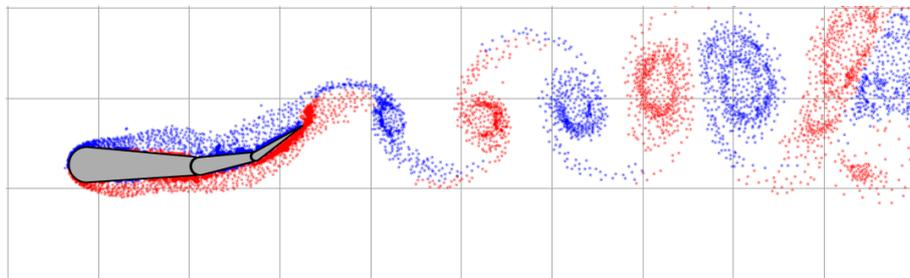
Figure.1 The vortex pattern around the self-moved fish-like foil
