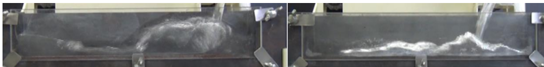
Fig.1 pouring experiment with water (left) and molten aluminum alloy (right).
