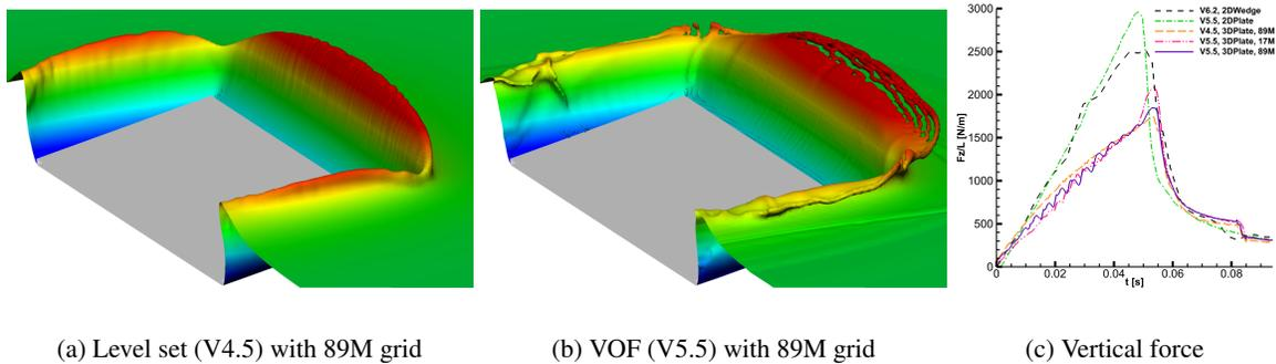
**Figure 1:** Vertical slam: free-surface and vertical force acting on the plate.
