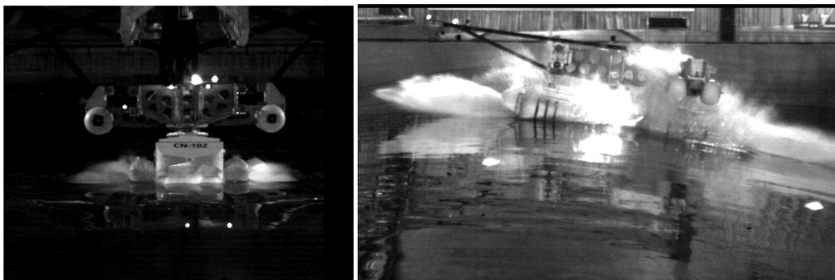
**Figure 1:** Impact of the mockup in waves
