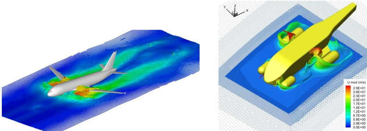
Figure 1. SPH simulation of airplane and helicopter ditching.
