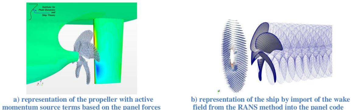
Figure 1: Illustration of the data exchanged in the coupling method
