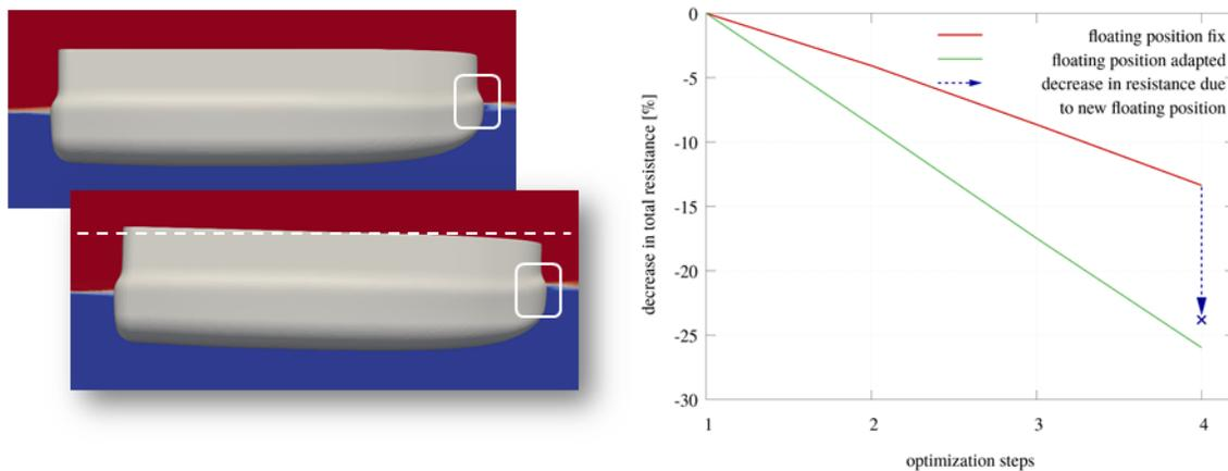
**Figure 1:** Comparison of frozen and free floating shape optimization with respect to resistance.
