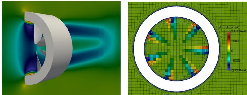
Figure 1: The left figure shows a RANS simulation of a transverse thruster. On the right the resulting immersed bodyforces can be seen.
