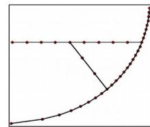
Figure 1: Lower part of the 2D half model of one cylindrical cross section.
