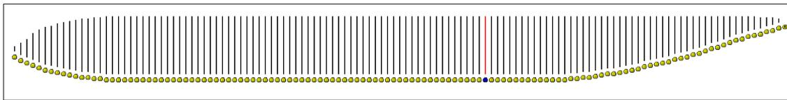
Figure 2: Fuselage Discretization in Sections. The hydrodynamic forces are evaluated on the submerged sections.
