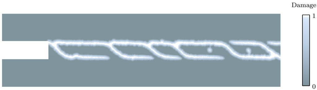
Figure 1: Shear failure mechanism for adhesive bond: final damage profile from a simulation with randomly located predefined defects
