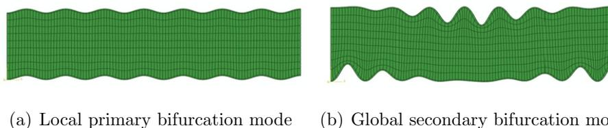
**Figure 1:** Typical post-critical response of a sandwich column under axial compression.
