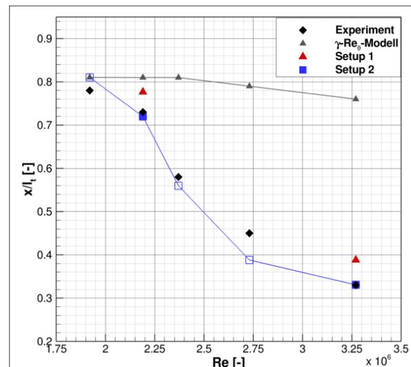
Figure 2: Transition positions on the NLF (2)-0415 profile; comparison of experimental and numerical results
