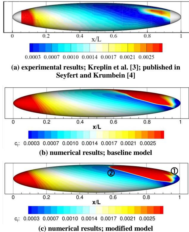
Figure 3: Comparison of experimental and numerical results on a 6:1 spheroid;  $Re = 1.5 \cdot 10^6$ ;  $\alpha = 5^\circ$
