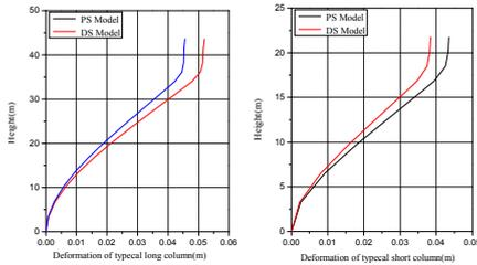
Fig. 3 Deformation of typical concrete columns of different models
