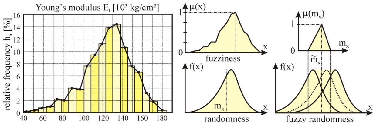
Figure 2: Relative frequency distribution of Young's modulus determined by 1546 ashwood samples [4] and possible models
