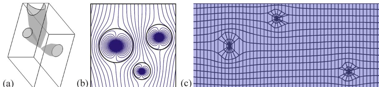
Figure 1: Wooden parts: (a) geometrical model, (b) computation of the fibre orientation and (c) automatic meshing procedure
