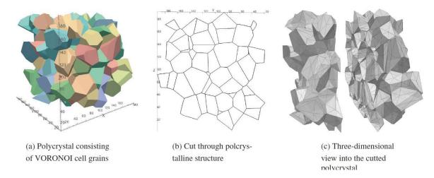
Figure 1: Polycrystal and discretization
