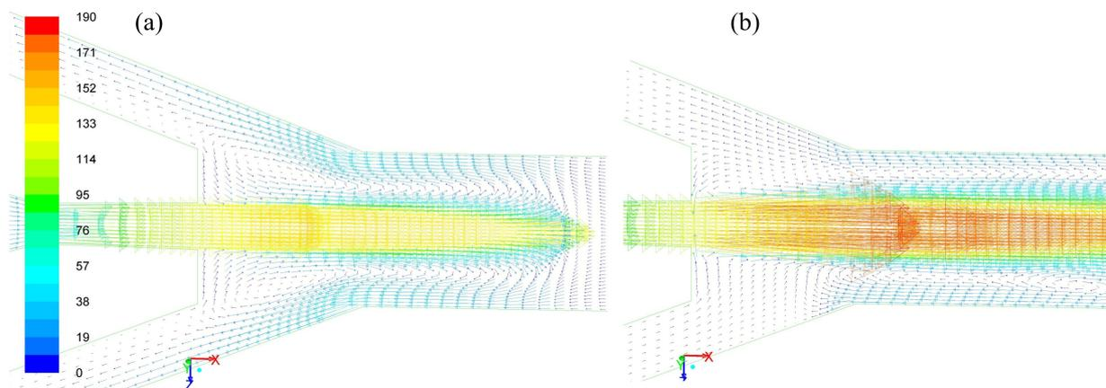
Figure 1: Velocity vectors for an ejector design working (a) incorrectly in typical cold ambient conditions and (b) correctly in typical hot ambient conditions.
