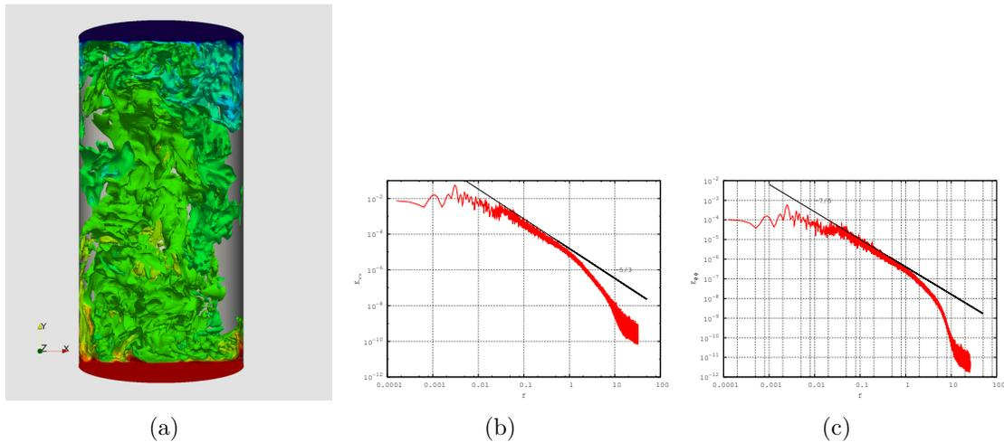
Figure 1: (a) Instantaneous flow configuration, (b) Energy spectra for the velocity fluctuations, (c) energy spectra for temperature fluctuations at  $r/H=0.25$ ,  $z/H=0.95$
