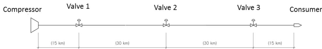
Figure 1. Configuration of the test-case with 3 valves
