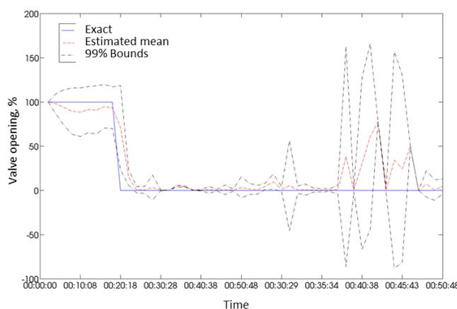
Figure 2. Detection of the closure of valve 1
