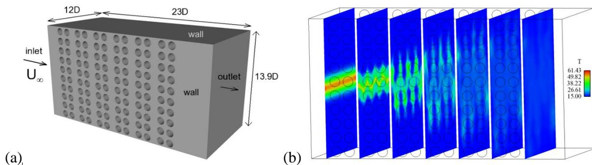
Figure 2: Specific industrial in-line tube bank: (a) Configuration of Jones et al. [4] (b) Mean temperature dispersion of Gaussian inlet spike using wall-modelled RSM.
