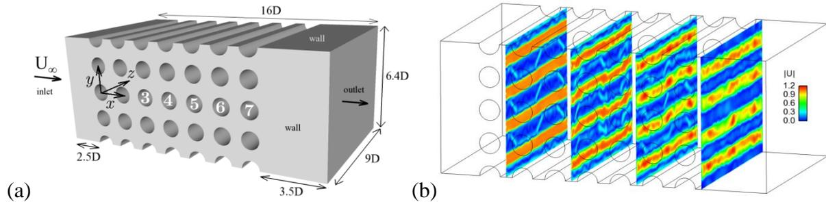
Figure 1: Generic in-line tube bank of  $P/D = 1.6$ : (a) Configuration of Aiba et al. [1] (b) mean velocity magnitude at various planes through the domain using the EB-RSM.
