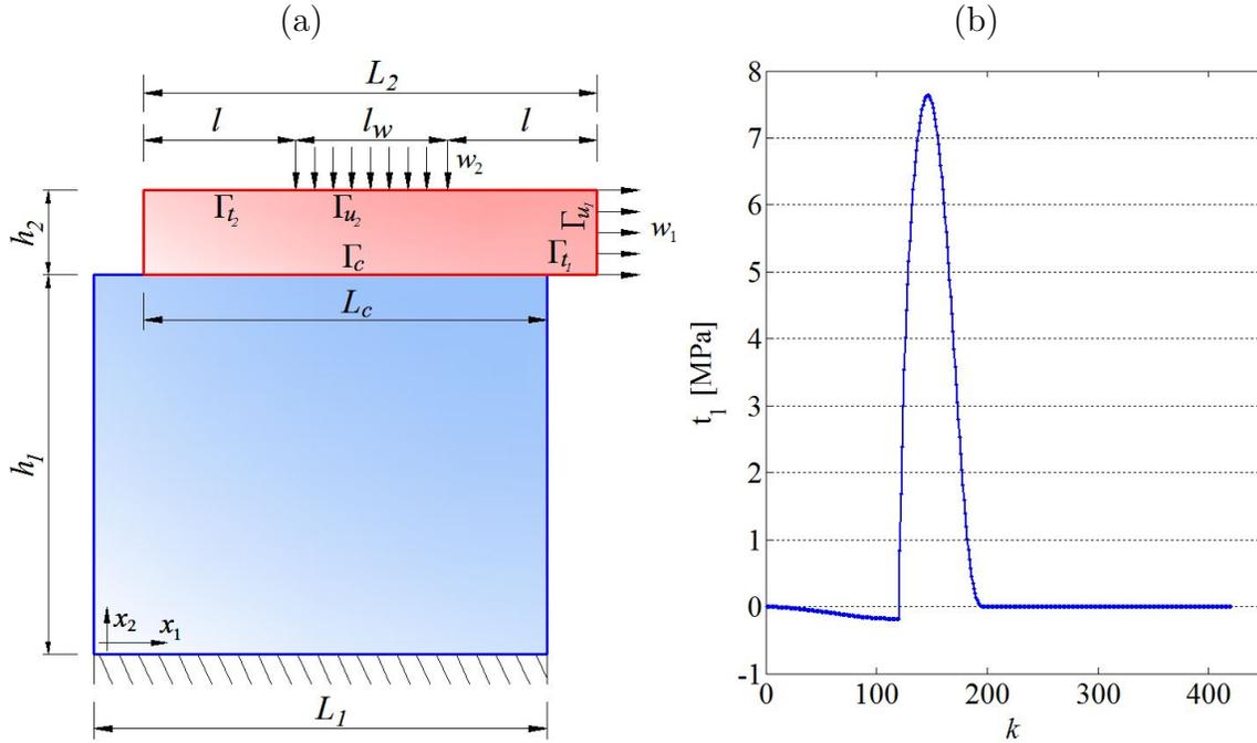
Figure 1: (a) Geometry of the multidomain contact model, (b) Distribution of stress  $t_1$  at load step  $k$ .
