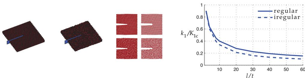
Fig. 1. Left: Regular and irregular 3D discrete meshes having single edge notches. Middle: close-up of deformations in a plane in the middle of the structure. Right: Normalized stress intensity at the tip vs. cell length/edge thickness ratio.
