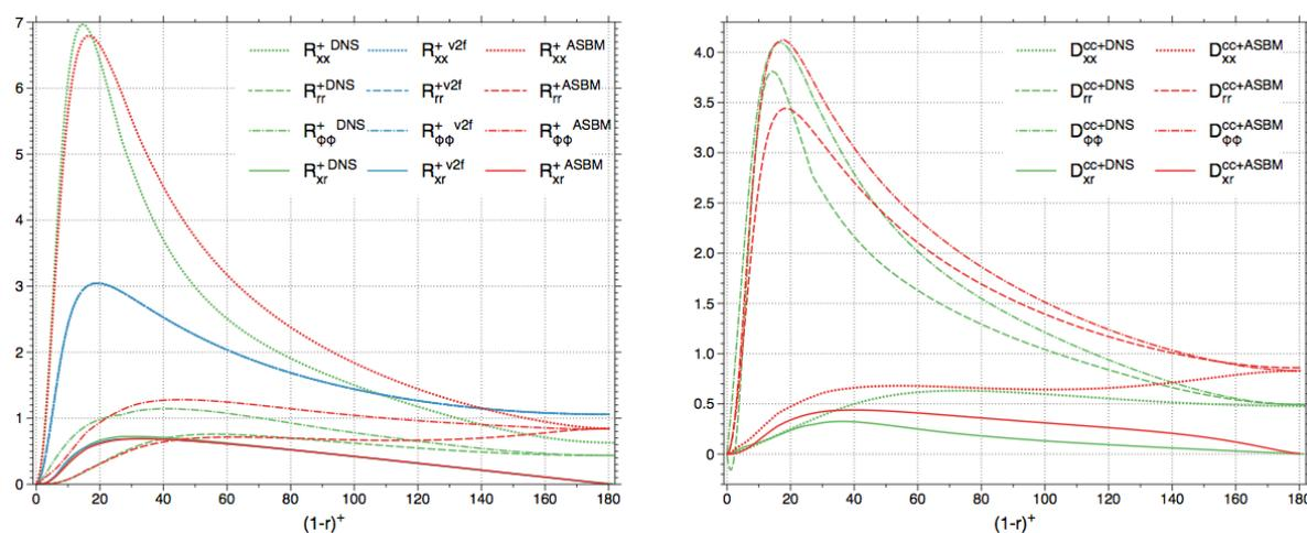
Fig[1]: Comparison between DNS, v2f and v2f-ASBM data, for the Reynolds stress (left) and homogenized dimensionality tensor (right).
