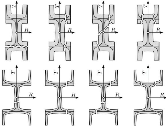
Figure 2: Failure mechanisms at single cell level for latewood (upper row) and earlywood (lower row) cells.
