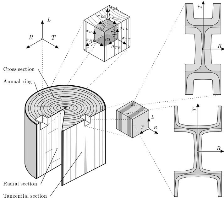
Figure 1: Multiscale approach for the determination of the global crack direction.
