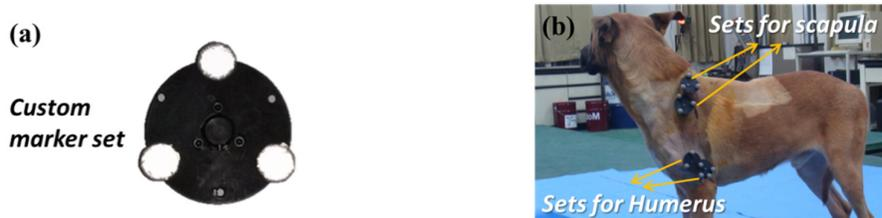
Fig 1. (a) A custom maker set with 3 balls, (b) Maker set installation in scapula & humerus
