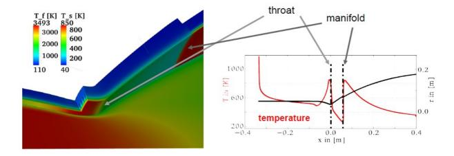
Fig. 1: Overview of the throat region of the subscale rocket thrust chamber. left: temperature in structure and hot gas;
