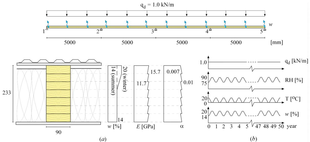
**Figure 1:** A glue laminated beam subjected to bending and cyclic moisture variation
