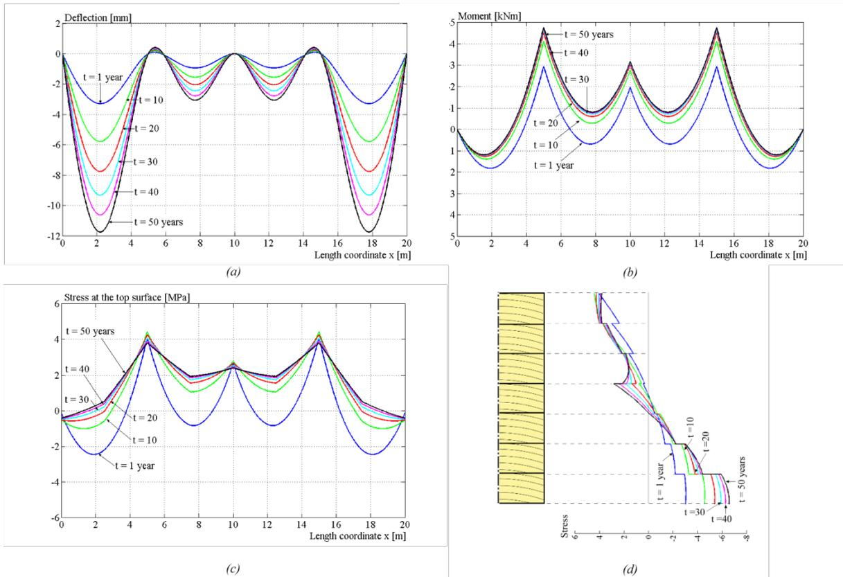
**Figure 2:** Numerical results at several (summer) times for the beam shown in Fig 1 (a) Deflection curves, (b) Moment curves, (c) Stress variation along the top surface, (d) Stress profile for the cross sections at supports 2 and 4.
