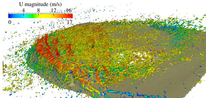
Figure 1: Iso-surfaces of the second invariant of the velocity gradient tensor  $Q$  colored with the velocity magnitude around the Bolund hill.
