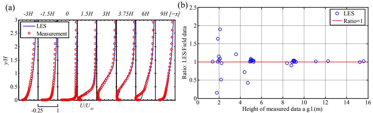
Figure 2: (a) Vertical profiles of mean wind-wise velocity compared with the measurements for flow over isolated hill at some longitudinal locations. (b) Ratio of LES results to field data for velocity magnitudes at different heights over the Bolund hill
