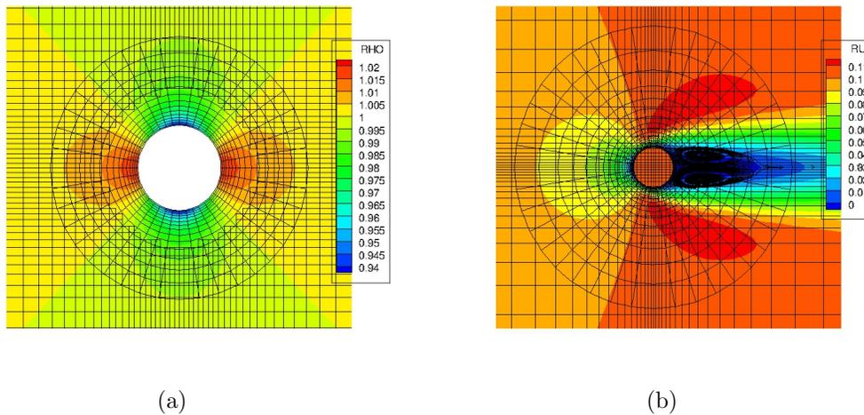
Figure 1: a) Density distribution of the Euler simulation, b) x-Momentum with the separation bubble of the Navier-Stokes simulation.
