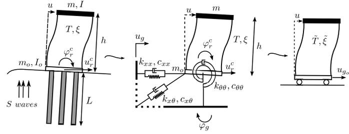
Figure 2: Substructuring model.
