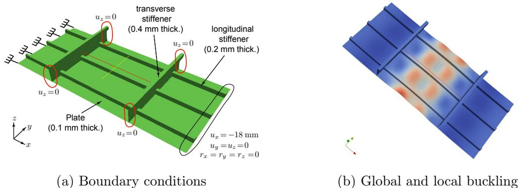
Figure 1: Stiffened pannel, representative of an aeronautical structure.
