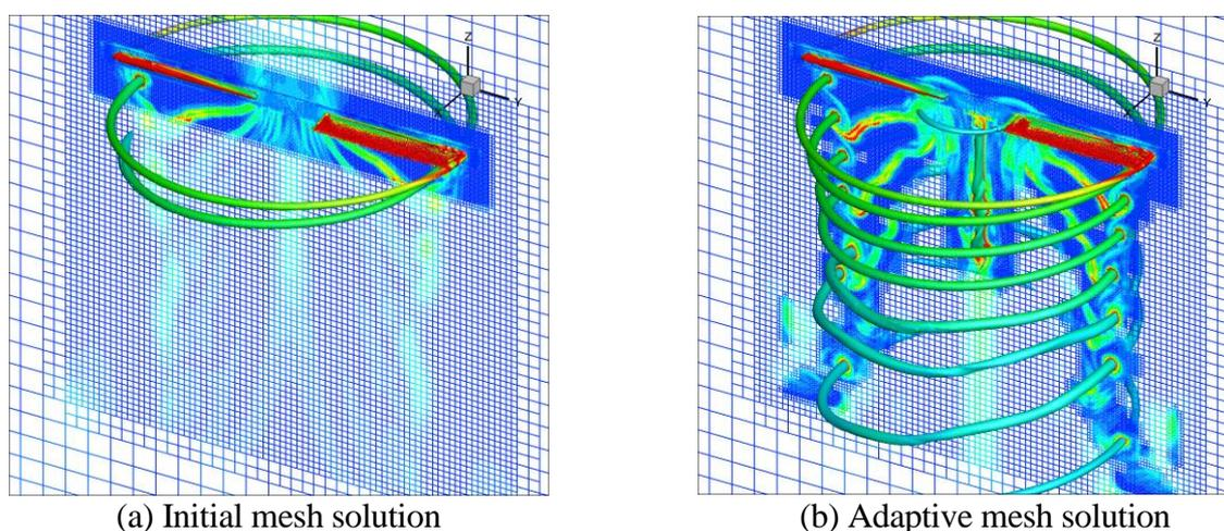
**Figure 1. Predicted wake structures for Caradonna-Tung rotor with 7<sup>th</sup>-order accurate method. (a) Initial mesh solution; (b) Adaptive mesh solution.**
