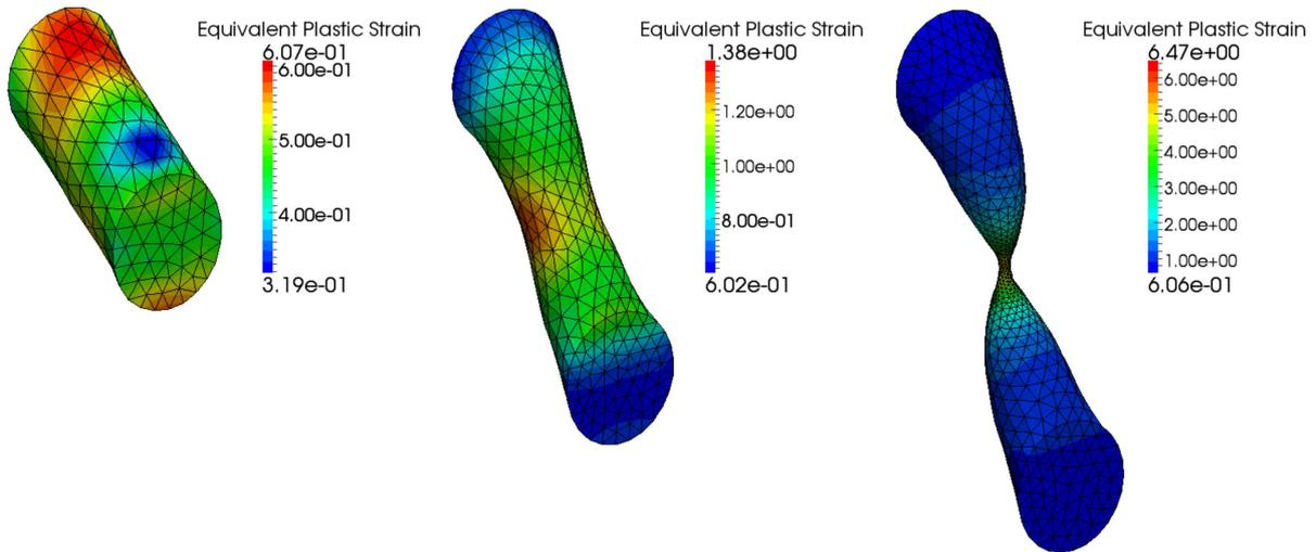
(a) 1.0 m displacement state with 3-times Mesh Rezonings    (b) 2.0 m displacement state with 7-times Mesh Rezonings    (c) 2.8 m displacement state with 12-times Mesh Rezonings
