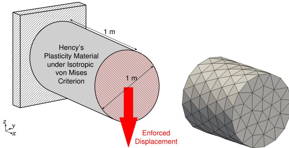
Figure 1: Outline of the shear necking analysis and the initial mesh. The material properties are 70 GPa Young's modulus, 0.3 Poisson's ratio, 100 MPa yield stress and 0.7 GPa constant plasticity coefficient.
