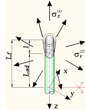
Fig. 1. Debonded extremity of a fibre under remote radial ( $\sigma_x^\infty$ ) and axial ( $\sigma_z^\infty$ ) stress.
