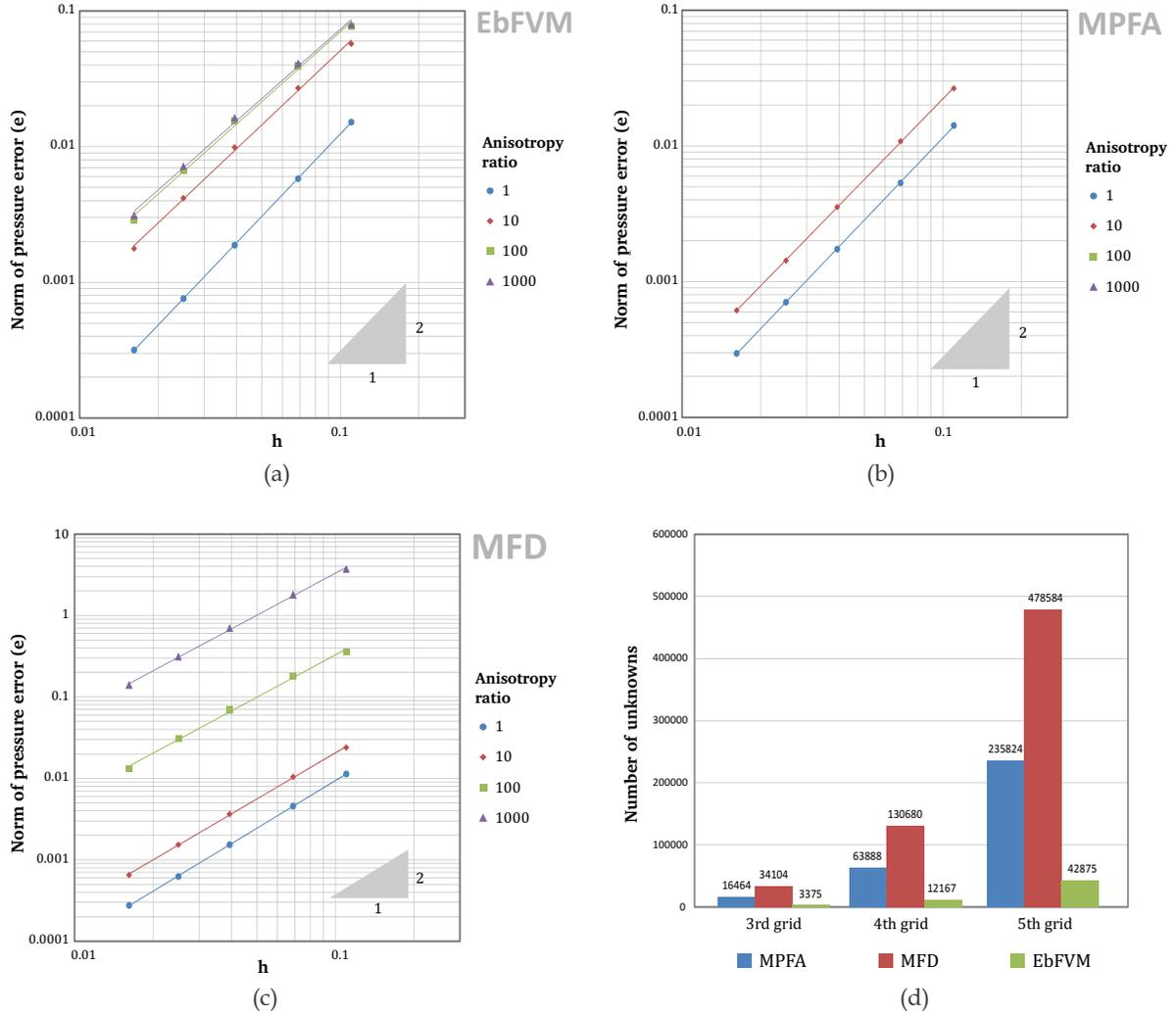
Figure 1: Convergence of pressure error on (a) EbFVM, (b) MPFA and (c) MFD. (d) Comparison of the number of unknowns solved in each method.
