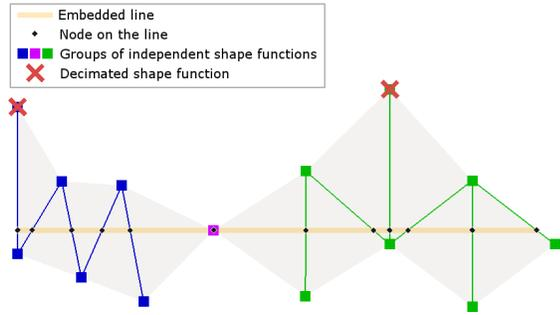
**Figure 2:** Reduction of the function space along a line: identify groups of independent shape functions and decimation.
