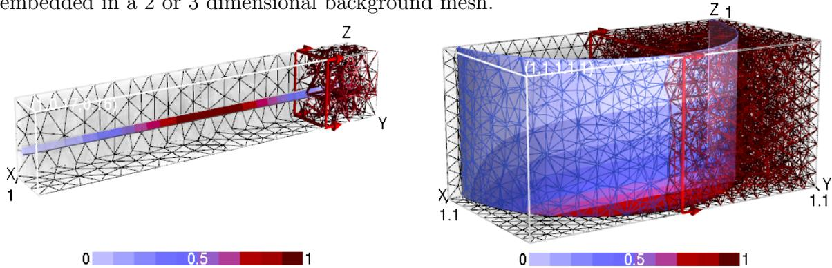
**Figure 3:** Embedded approximations along a line (left) and a surface (right) to the solution of thermal problems over 3D meshes.
