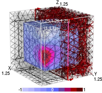
**Figure 1:** Solid under thermal loading: 1D Dirichlet boundary condition.
