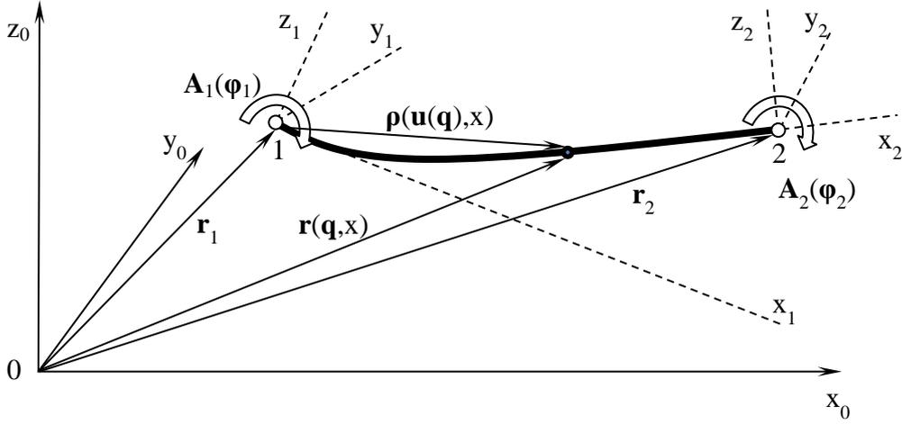
Figure 1. Geometry and generalized coordinates of a single beam element.
