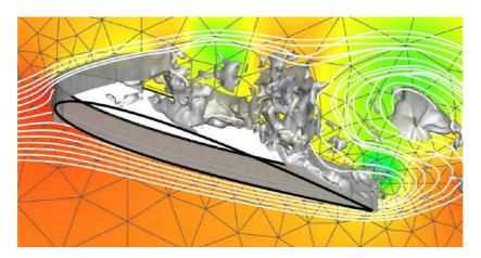
Figure 1: Implicit LES high order DG-Fourier solutions aft a three dimensional NACA0012 at Re=10000 and AOA=20° using polynomial order 5 and 16 Fourier planes.
