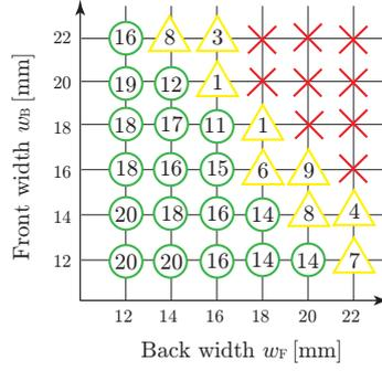
Figure 2: Number of buckling modes for Model 1 at  $g = 10$  [mm]
