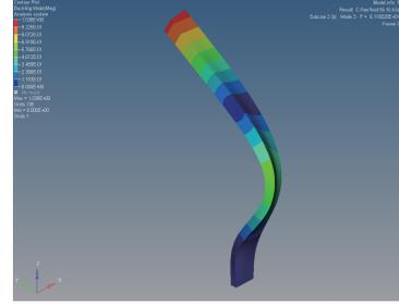
Figure 3: 2nd Buckling mode shape for Model 1 at  $g = 10$  [mm]
