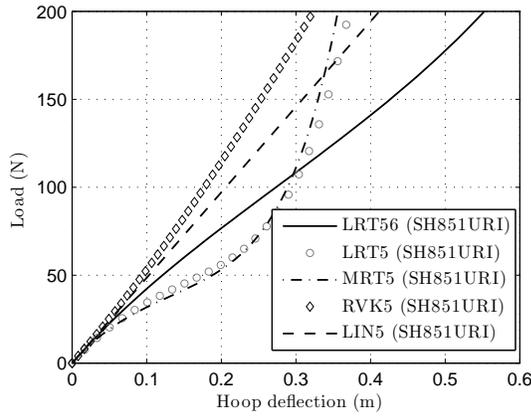
Figure 2: Static response of the hoop deflection under a concentrated force in hoop direction
