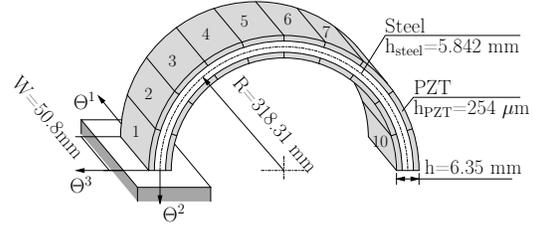
Figure 1: PZT laminated semicircular cylindrical shell
