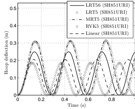
Figure 3: Dynamic response of the hoop deflection under a step tip force of 50 N
