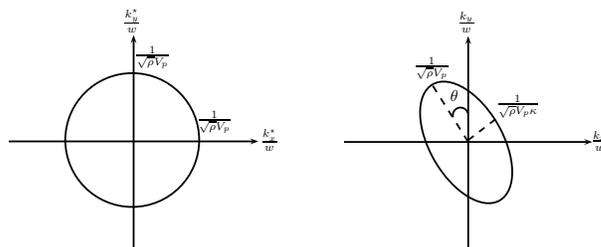
**Figure 2:** Slowness curves of isotropic (left) and elliptic TTI (right) cases – for 2D P-waves
