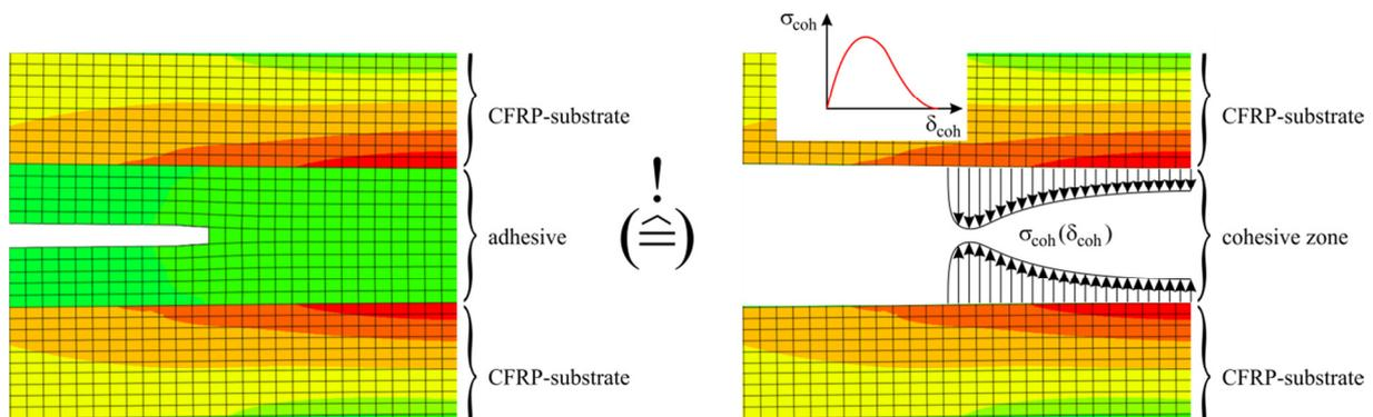
Fig. 1: Homogenization approach for determination of cohesive zone parameters.
