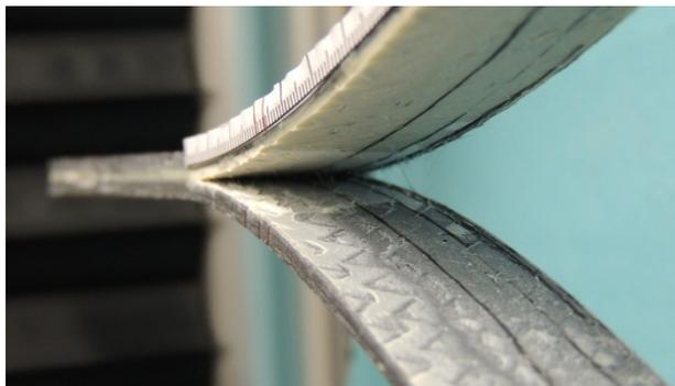
Fig. 2: Mode I fracture mechanics experiment on adhesively joint CFRP sample.
