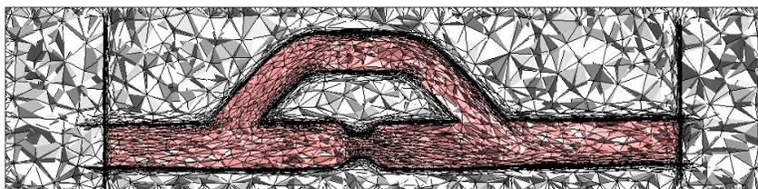
Figure 2: Anisotropic mesh adapted to the geometry and to the solution for blood flow through a bypassed artery at Reynolds number  $Re = 500$ .
