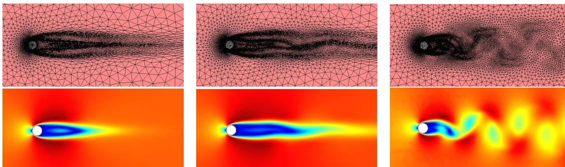
Figure 1: Transient mesh adaptation and visualization of corresponding solution for flow over 2D cylinder at  $Re = 100$ .
