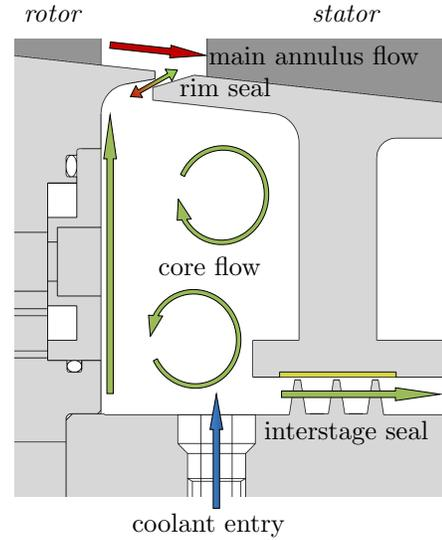
Figure 1: Flow structure in rotor stator cavity of axial two-stage turbine rig
