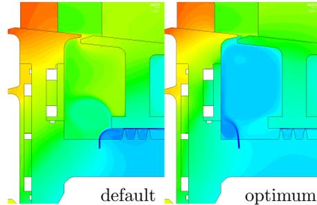
Figure 2: Temperature field at default and optimal configuration
