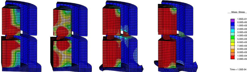
**Figure 1:** Different states of torsional transducer at instants  $t = 9, 18, 117, 135 \mu s$ .
