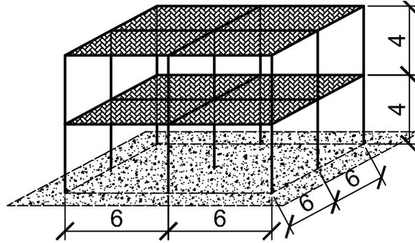
Figure 1: Structural model taken into consideration.
