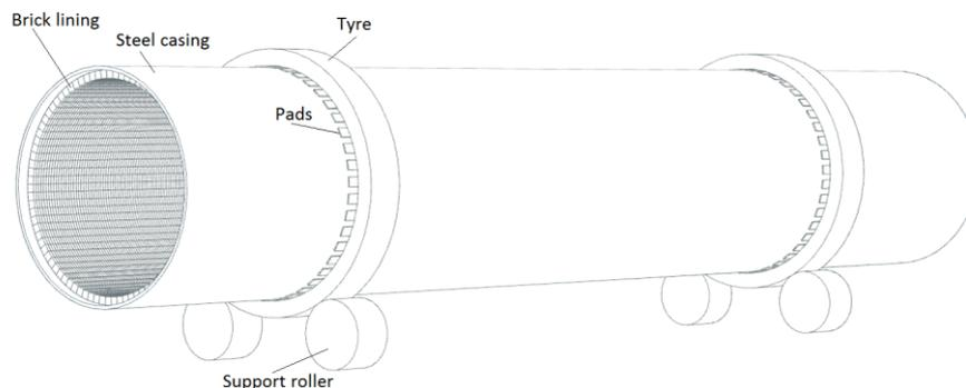
Figure 1. Illustration of a typical short dry-kiln used in iron-ore pellet industry ( $D_{\text{outer}}=7$  m,  $L=40$ m).
