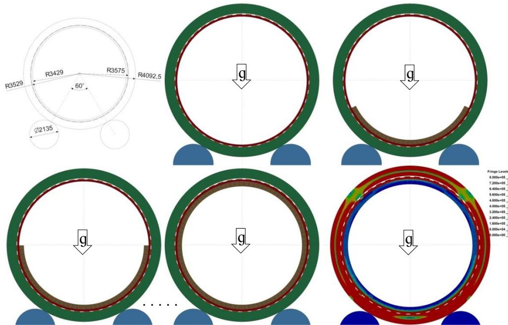
Figure 3. Illustration of the bricklaying sequences using the finite element method.
