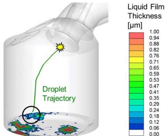
Figure 2: Trajectory of a separated droplet until pre-ignition timing (yellow sign)
