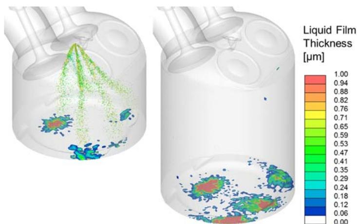
Figure 1: CFD-simulation result of the injection and wall film formation
