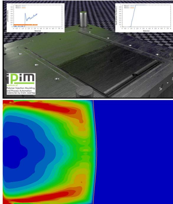
**Figure 1:** Mold filling simulation and polymer conversion of a flat plate geometry
