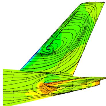
Figure 2: Friction lines on the VTP for an URANS study with  $C_p$  contours (no rudder deflection, no sideslip angle).
