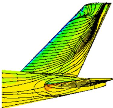
Figure 1: Friction lines on the VTP for a RANS study with  $C_p$  contours (no rudder deflection, no sideslip angle).
