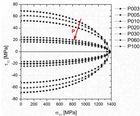
**Figure 2.** Failure envelope evolution with manufacturing pressure.
