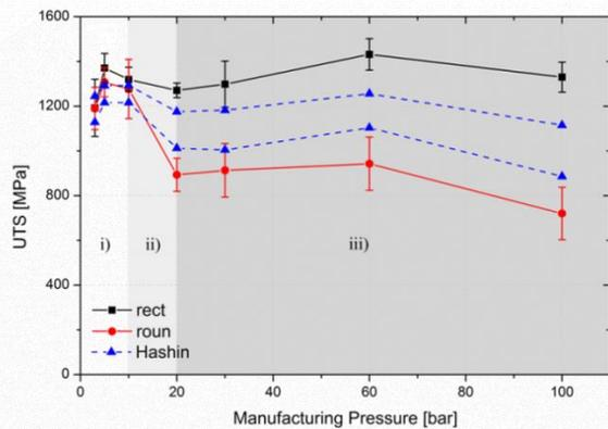
**Figure 1.** SLJ strength dependence on the manufacturing pressure.
